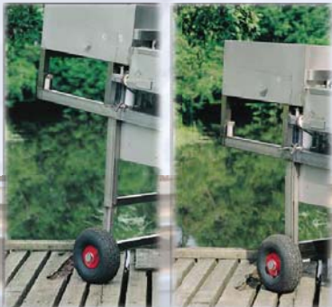
Rear end is height-adjustable
